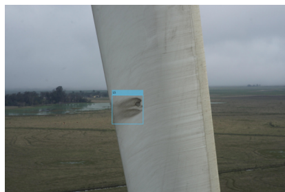
(e) Lightning Strikes the receptor and a portion of the blade
